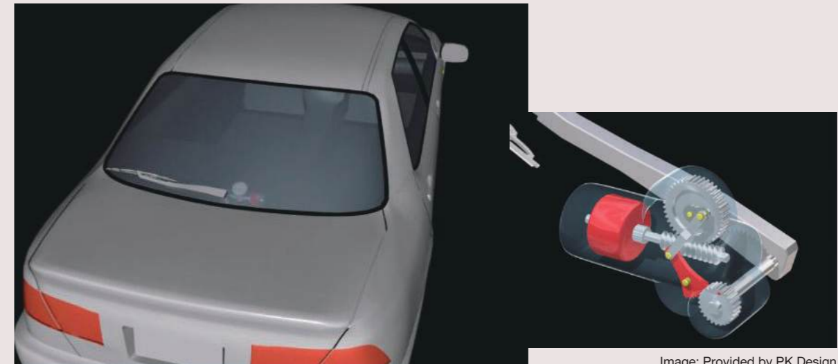
Worm gear used for the oscillating mechanism of wipers
