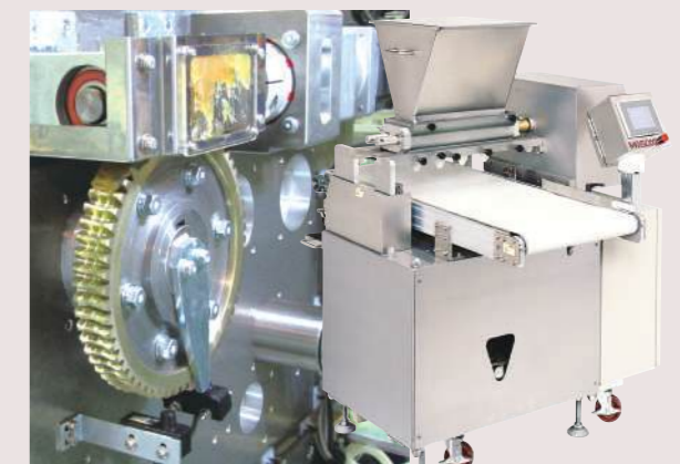
KWGDL Duplex Worm Wheels and AGDL Worm Wheels used for indexing and driving, for accurate filling of a fixed amount of ingredients
