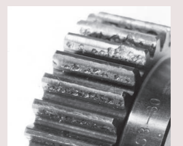
Example of wear due to insufficient surface durability
