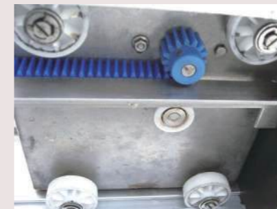
PR plastic rack used for feeding Long Strip Cutter
