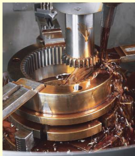
Gear cutting by CNC Gear Shaper
