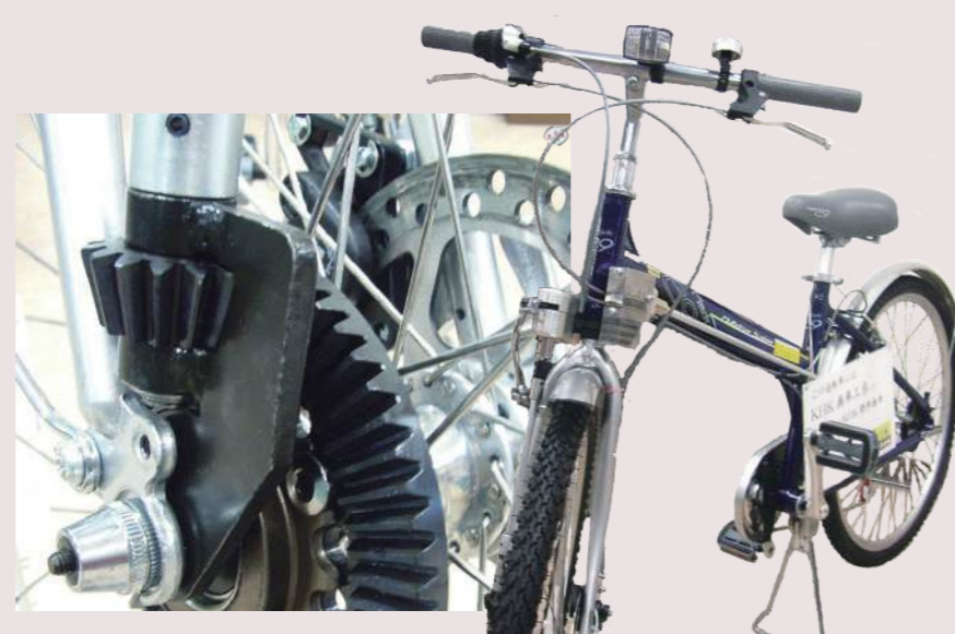
SB Bevel Gears are used in the driving components in both the front and rear wheels
