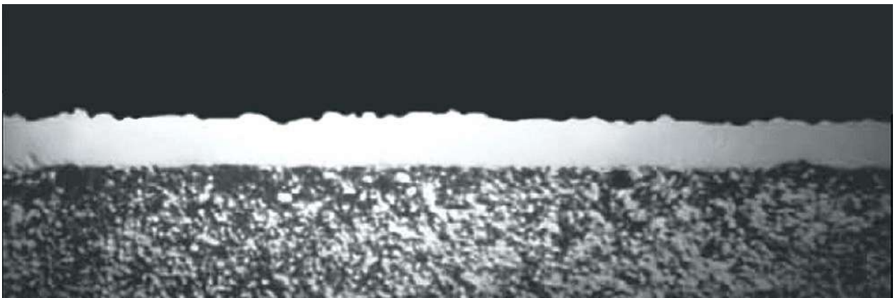
ATCoat coating surface (microscopic view)
